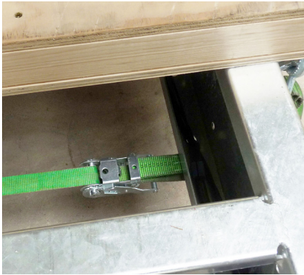
Base plate secured to frame with tensioning straps
