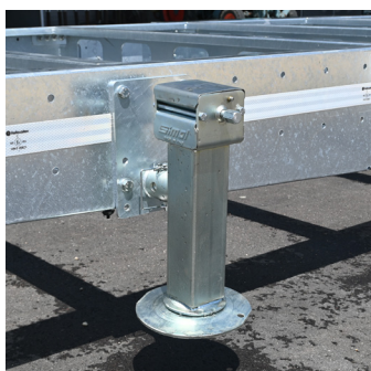
Crank supports in driving position (left) or retracted (right)
