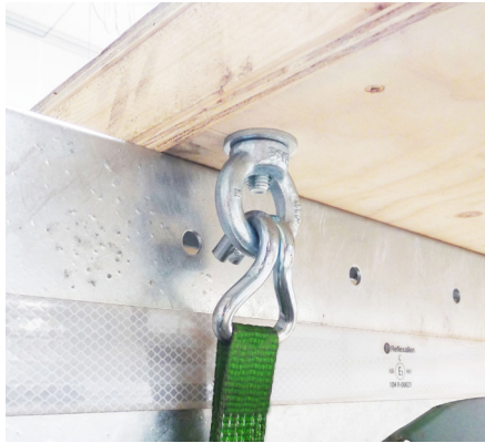
Lashing eye for 350 daN lashing force anchored in the base plate
